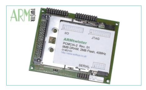
The **ARMtwister** is a small embedded control board with PCMCIA socket utilizing the Atmel AT91M40800 Microcontroller. With its customized version of uClinux-2.4 it is possible to use IEEE 802.11 Wireless PCMCIA cards, as well as Ethernet cards and most other 16-bit PCMCIA cards.
